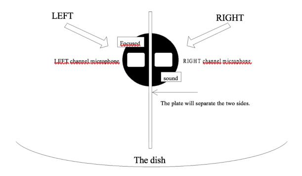
**STEREO MK3:** The plate separates the two sides from each other, while the focused sound will affect the two microphones equally **Result:** the focused sound will be recorded mono, while the background will be <u>presented</u> in stereo, to L&R channels. NOT M/S! (3 channels)
